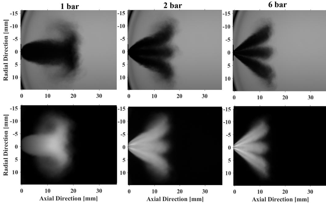
Figure 3: Ensemble averaged image of propane spray structure at  $350 \mu\text{s}$  ASOI for different CVC pressures shown at the top of the figure; DBI images are shown in the top row, and Mie-scattering below. The spray liquid length is measured by taking the maximum axial length of the spray edge (dark region for DBI images or the gray region for Mie-scattering images) of individual spray images (not shown here).
