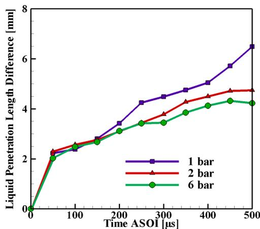
Figure 5: Liquid length measurement difference between DBI and Mie-scattering technique
