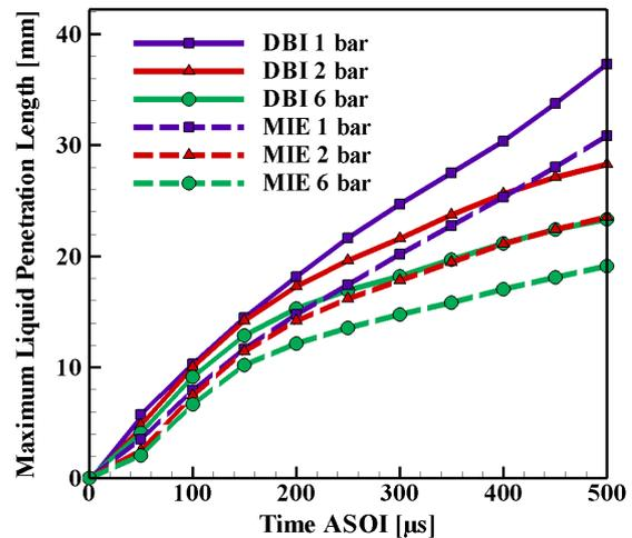
Figure 4: Comparison of maximum liquid penetration length profiles using Mie-scattering and DBI
