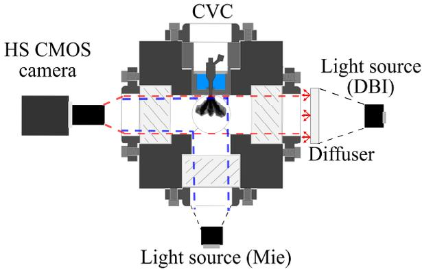
Figure 1: Schematic of the CVC and each imaging technique; note that the DBI and Mie-scattering experiments were conducted separately
