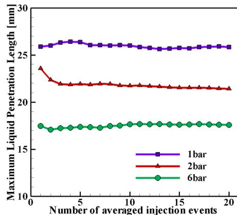
Figure 2: Ensemble-averaged liquid penetration length with a varying number of injection events used in the averaging
